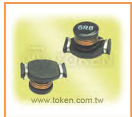
TPU1813DHP rugged self-leaded construction with advance wire wound technology enables large current, lower DCR, and less than 5.0mm height. It is ideal for high power DC-DC applications. Inductance values for the TPU1813DHP are from 0.18  $\mu$ H to 100  $\mu$ H with rated current up to 14 A.
