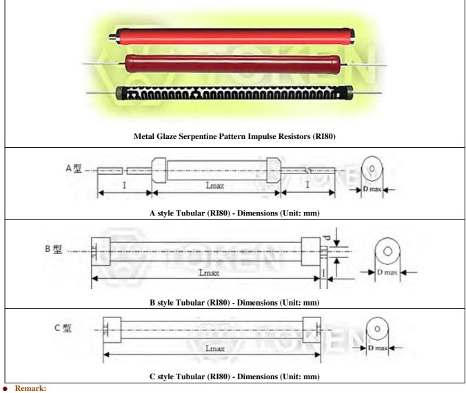
Rated continuous Working Voltage (RCWV) shall be determined from RCWV =  $\sqrt{\text{Power Rating} \times \text{Resistance Value}(\Omega)}$ When RCWV ≥ Max. Working Voltage listed above, RCWV = Max. Working Voltage.
