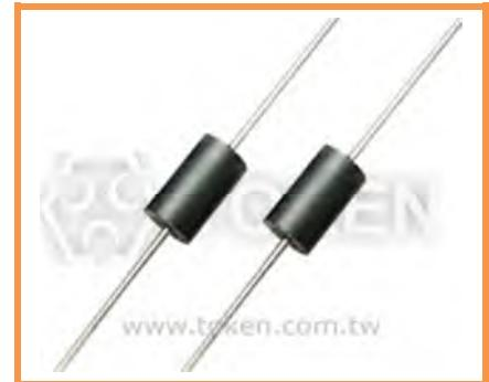
By comparing with traditional inductors, Token's (TCFB) has better high-frequency filter characteristics. Ferrites at high frequencies showed resistance characteristics at high frequencies, equivalent to a low inductor quality factor, it can be quite a wide frequency range, to maintain high impedance, thereby enhancing the effectiveness of high-frequency filter.
