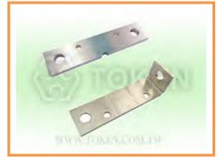
This is a new Bus-Bar Battery Shunt resistor that has rated voltage drop 75 mV capability with 1.5 m $\Omega$  to 0.075 m $\Omega$ . Specifically, it is possible to output 75 mV from the voltage terminal with a current from 50 A to 1000 A with precision  $\pm 0.5\%$  and  $\pm 1\%$  tolerance in option.
