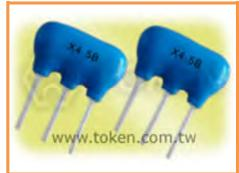
In TV set, video signal is used in picture amplitude circuit after video signal detection block, ceramic resonator is inserting here and trap circuit is formed in order to eliminate sound signal involved in video signal.
