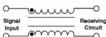
Use Common Mode Choke Between Signal Lines
